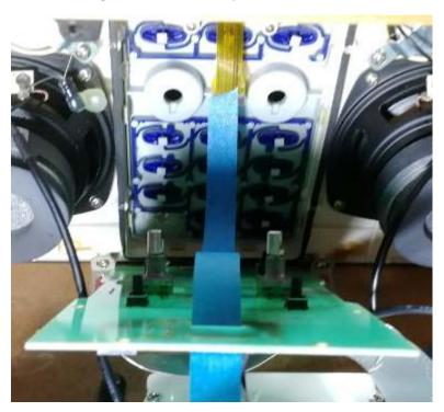
7. Connect the display cable. I used 2 toothpicks in the small holes of the display cable (see image) to move it up into position and then move the clamp up to secure it. Fold the small black cover back over the cable.
