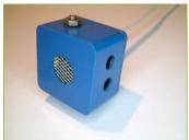
A terminal block carried the connections to the vehicle and the thermistor was housed in the smallest plastic box I could find: problem was, it needed to sense the outside airflow (eg behind the front bumper), so it needed holes to check the airflow, but it needed to be kept dry at the same time.....
