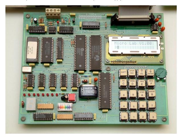
^^ My Teach-In 93 Micro Lab up and running, powered by my Mini Lab. The LCD could be backlit with an EL panel (via two pads on the right hand edge); the green control adjusted LCD contrast. Keith included a comprehensive Micro Lab manual and provided readers with laser-printed keycap legends.
