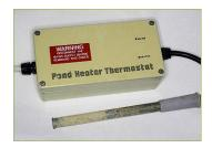
I had a small fishpond containing a wide range of ornamental goldfish and some cute Shubunkins, and I used a floating mains electric heater to keep a small area clear of ice during the wintertime freeze-over. This allowed noxious gasses from decomposing materials to escape and allowed oxygen in as well. Rather than keep the thing permanently powered on, I hit upon the idea of using thermostatic control and I chose another favourite National Semiconductor chip, the LM3911 for
