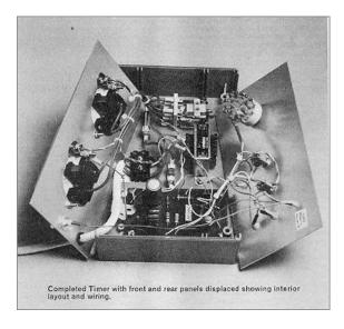
Apart from fiddling with the circuit, which itself was pretty basic, I spent much of the time working on the appearance and style of the prototype. It was built in a large Verobox in light/ dark ABS with attractive anodized aluminium panels. I chose a spun aluminium knob to match, and to mimic a clock
