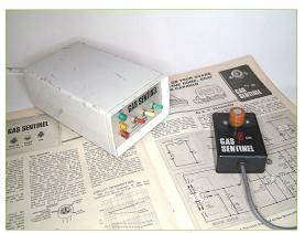
One of my favourite constructional projects, this gas leakage detector used a Figaro TGS813 sensor with a simple op.amp acting as a comparator. The circuit was very simple, so any hobbyist could build it, and it triggered a thyristor and a transistorised buzzer to warn of a rise in gas levels.
