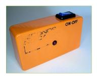
This project was also intended for my "Uniboards" series but it was published on its own, as it didn't fit into IPC's prescribed format of standard-size veroboard. It was just a transistor astable multivibrator that flashed an I.e.d., which could be fine-tuned to produce one flash per second. What use was that? Well not much really, until IPC rechristened it as "Darkroom Timer" which made more sense.
